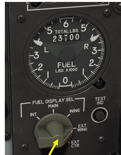
Fuel Quantity Display Selector Internal/Main/Wing/External Wing/External Centerline
