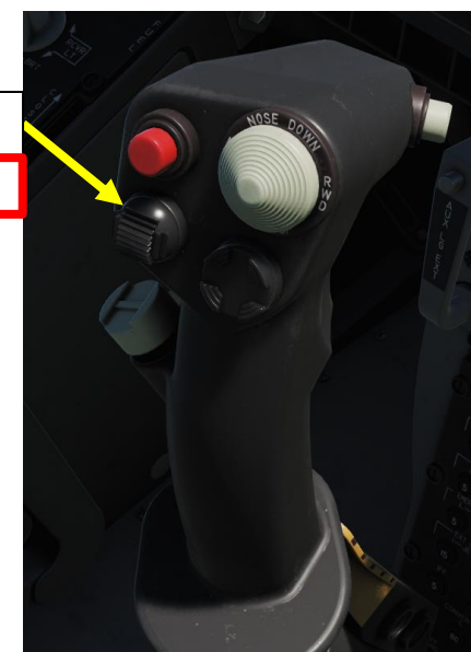
TMS (Target Management System) Switch
