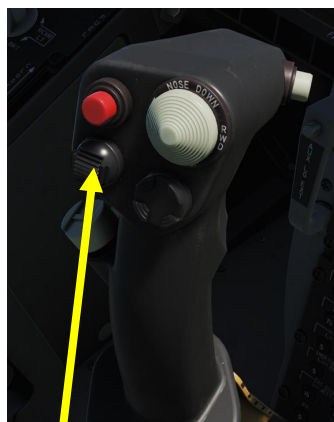
TMS (Target Management System) Switch
