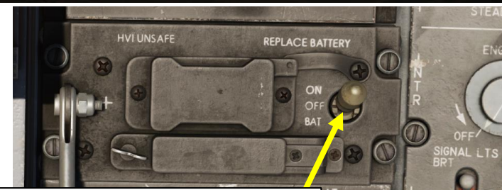
Scorpion HMCS (Helmet-Mounted Cueing System) Power Switch • ON (FWD): Power to the HMCS through the aircraft electrical power supply system
