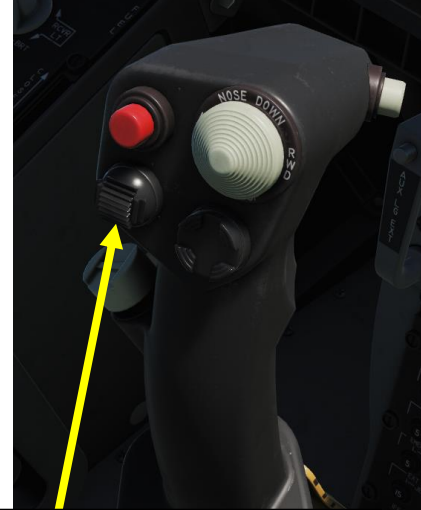
2 TMS (Target Management System) Switch
