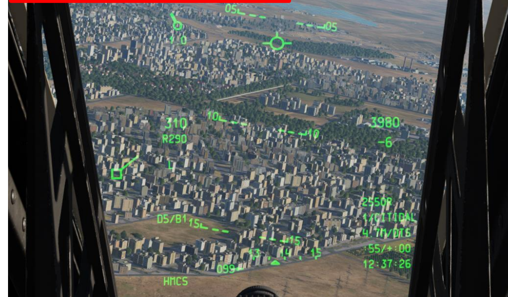
HMCS Crosshair, Own SPI and HDC ON
