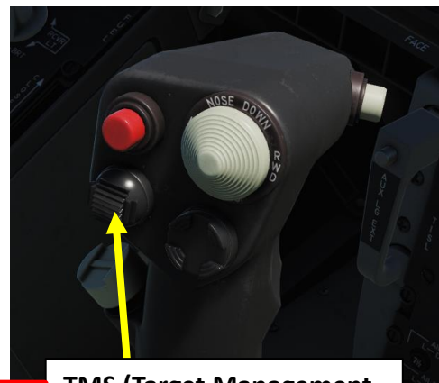
8 TMS (Target Management System) Switch
