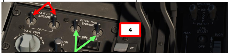
SAS (Stability Augmentation System) PITCH CHANNEL ENGAGE Switches
