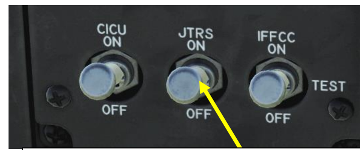
JTRS (Joint Tactical Radio System) Power Switch
