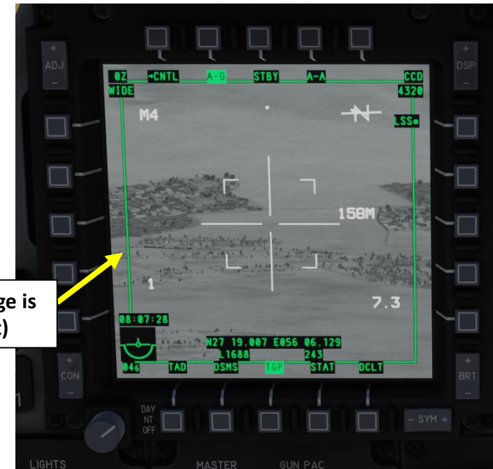
SPI Sensor Indicator TGP: Current Sensor Point of Interest (SPI) is from Targeting Pod
