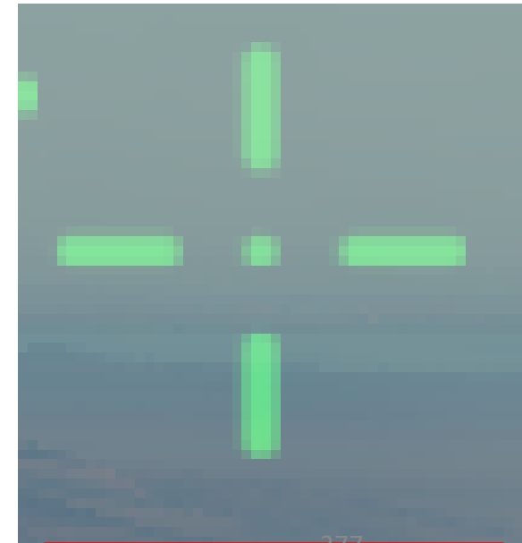
4000 ft Wind Corrected Cross Reticle
