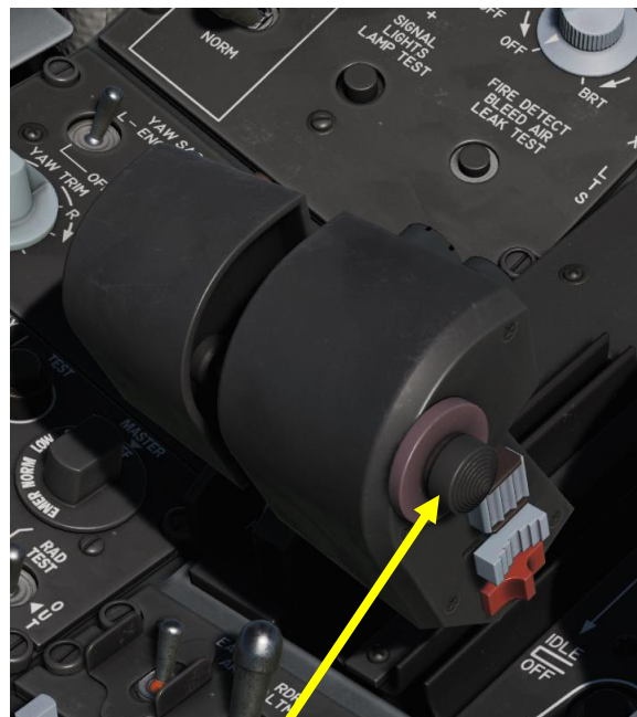
Microphone Switch • FWD: Transmits on VHF Radio 1 (AM) • AFT: Transmits on VHF Radio 2 (FM) • DOWN: Transmits on UHF Radio
