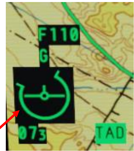
ARS (Attitude Reference Symbol) Shown: 45 deg dive, banking slightly right, altitude 7300 ft
