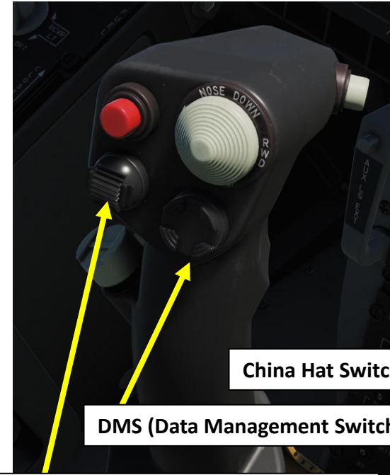
TMS (Target Management System) Switch
