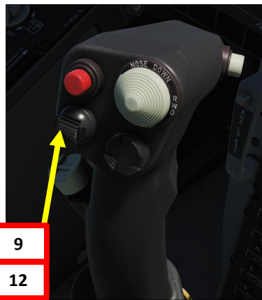
TMS (Target Management System) Switch
