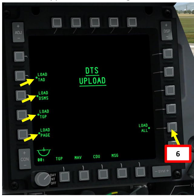
6) Click on "LOAD ALL" OSB on the right to reload all DSMS stations. Reload is complete when asterisks appear next to every menu.
